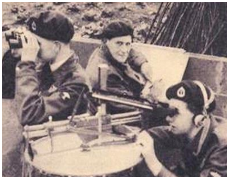
A Post Instrument plotter, with a Mickelthwaite height adjuster attachment, used to plot aircraft.
